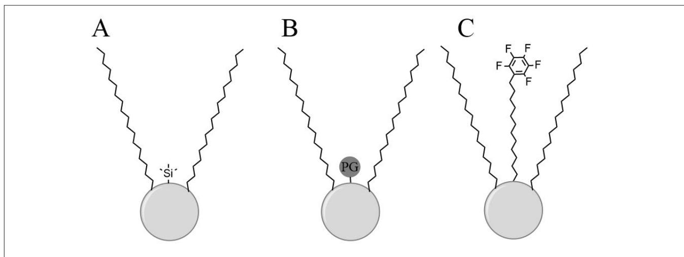
Figure 2. Schematic representation of phase chemistries A) C18 phase, B) AQ and AQ Plus phase where PG = Polar End capping, C) C18/PFP phase.
