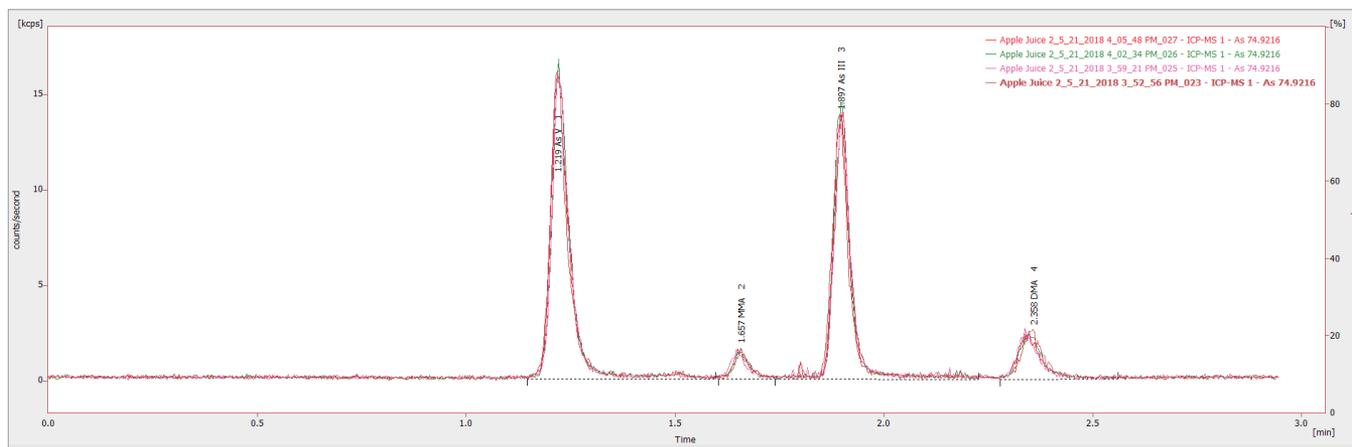
Figure 3. Chromatogram showing four injections (20  $\mu\text{L}$ ) of an undiluted apple juice sample from different sample vials.
