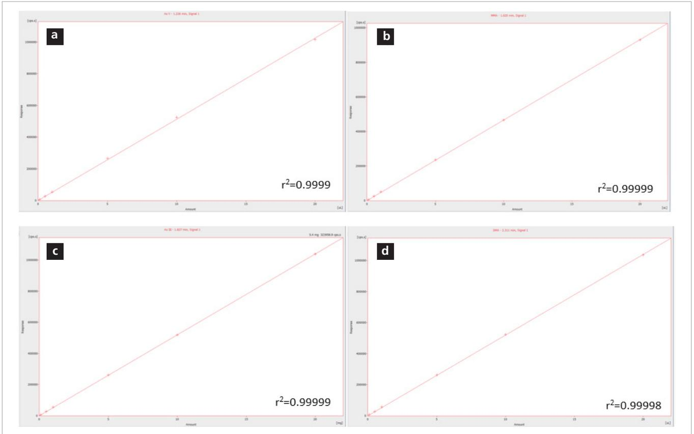
Figure 1. Linear regression of calibration standards ranging in concentration from 0.1-20 µg/L for (a) As V, (b) MMA, (c) As III, and (d) DMA in the mobile phase (pH 4.0) and the respective correlation coefficients.
