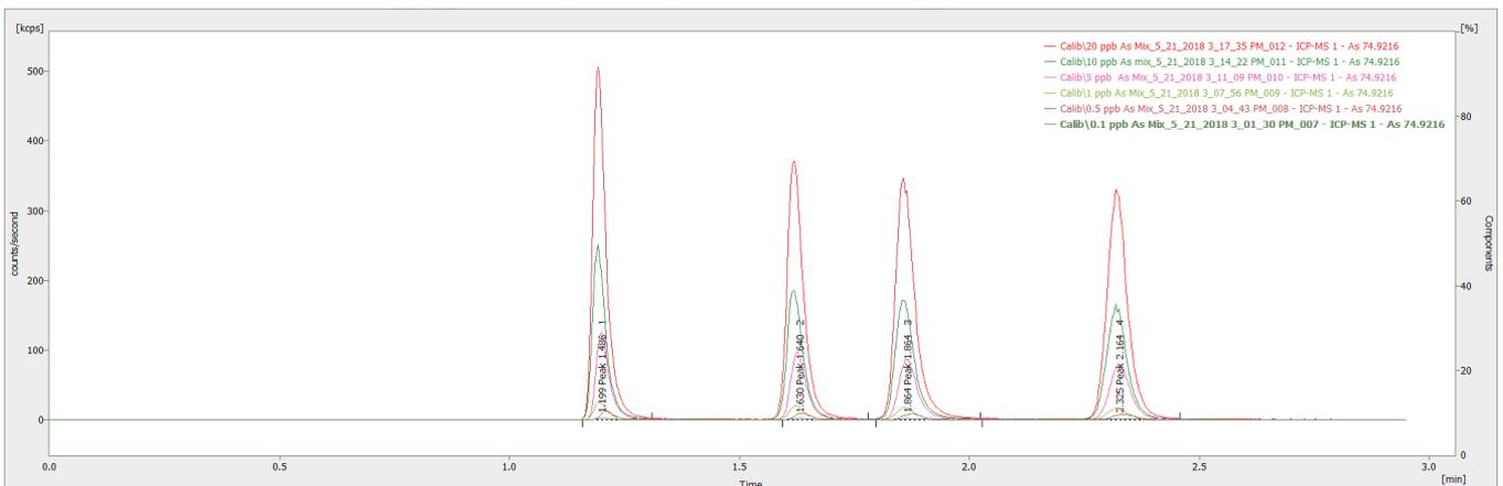
Figure 2. Chromatogram showing overlay of calibration standards (0.1 – 20 µg/L) in the mobile phase at (pH 4.0).
