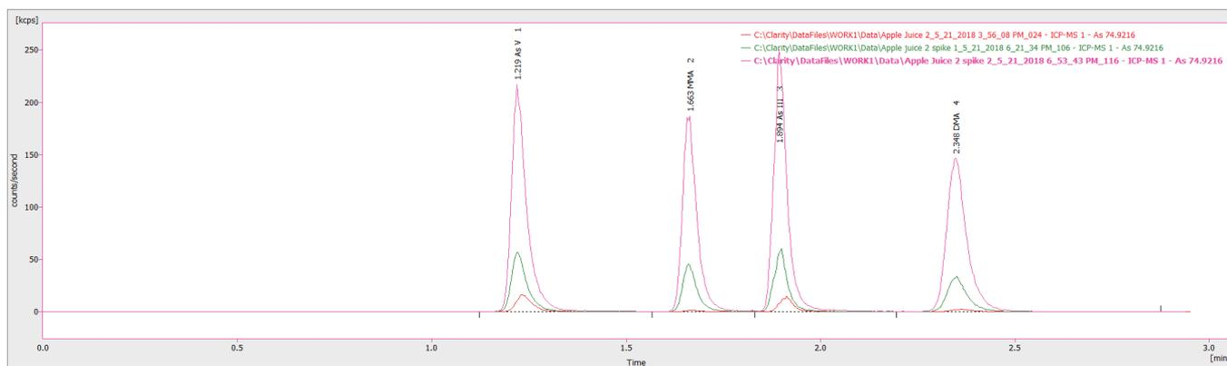
Figure 4. Chromatogram showing an undiluted apple juice sample as well as low-end (2  $\mu\text{g/L}$ ) and high-end (10  $\mu\text{g/L}$ ) spikes of this sample.
