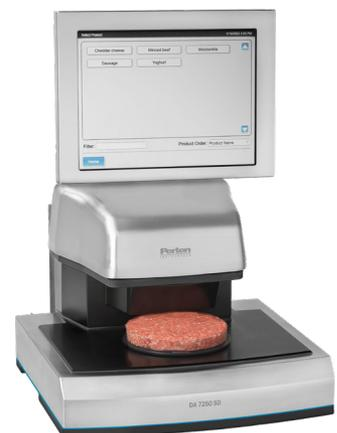
As samples are analyzed in open cups, or even disposable petri dishes, no or minimal cleaning is required and there is no risk of sample cross-contamination.
