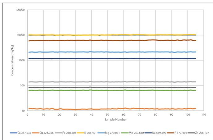
Figure 2. Three-hour stability run of turkey feed.
