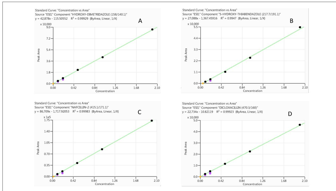
Figure 3. Calibration curves for hydroxyl-dimetridazole (A), 5-hydroxy-thiabendazole (B), nafcillin (C) and dicloxacillin (D) obtained from standards prepared in chicken sample matrix (analyte concentrations range from 0.1X to 2X).
