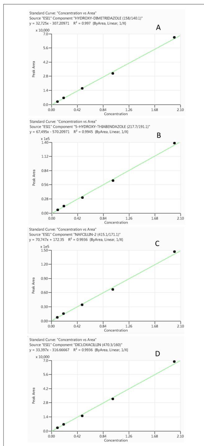
Figure 2. Calibration curves for hydroxyl-dimetridazole (A), S-hydroxy-thiabenzazole (B), nafcillin (C) and dicloxacillin (D) obtained from standards prepared in reagents only (analyte concentrations range from 0.1X to 2X).
