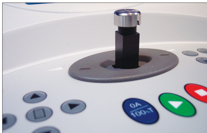
Figure 3. Close-up TrayCell™ in the LAMBDA Bio+.
