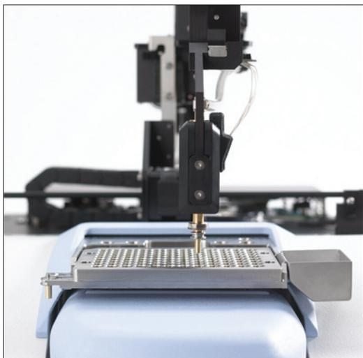
Figure 2. DSC 8000/8500 with autosampler.
