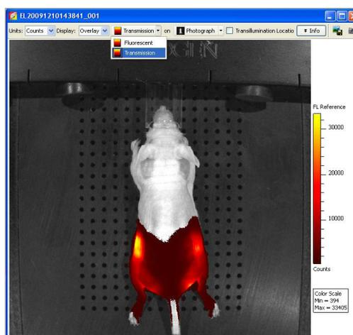
Figure 1. Attenuation map created by excitation Neutral Density (ND2) filter/emission 620 nm
