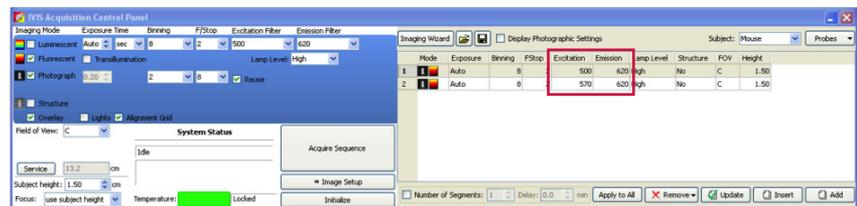
The selection criteria above assume that you are using the IVIS Spectrum, Lumina II, XR, or Kinetic with the numbered filters. If you have the IVIS Lumina, Lumina II, 50, 100 or 200 with the standard filter wheel, simply select the labeled background (BKG) filter that corresponds to the specific filter which you selected. For example, specific filter pair **Ex. DsRed/Em. DsRed** – autofluorescent background filters **Ex. DsRed BKG/Em. DsRed**.
