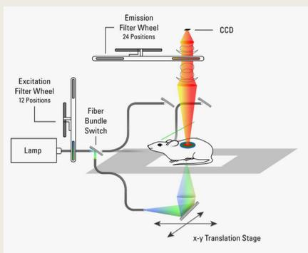
Figure 1. Fluorescence tomography instrumentation. The fluorescence tomography source-detector geometry in this work is such that excitation light is directed into the animal by a 2 mm diameter beam from underneath the animal bed (green/blue beam). The continuous wave fluorescence (red/yellow beam) is imaged through emission filters at the CCD.
