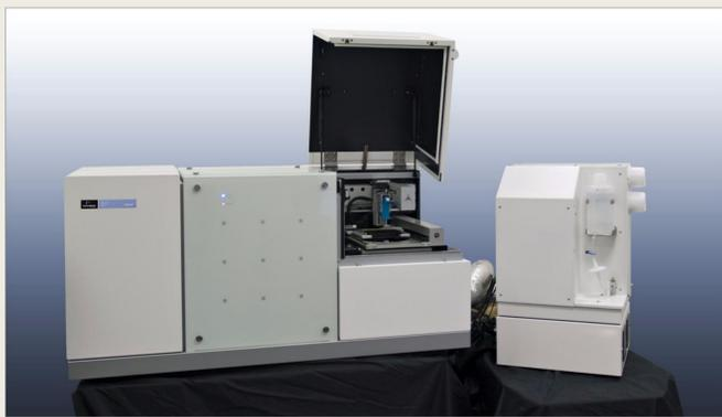
Fig. 1 | Opera™ platform with Environmental Control Unit (ECU)
