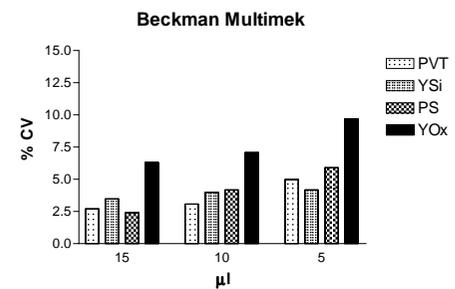
Figure 3. Precision achieved when dispensing [<sup>3</sup>H] labelled beads into a 384 well plate using the Beckman Multimek.
