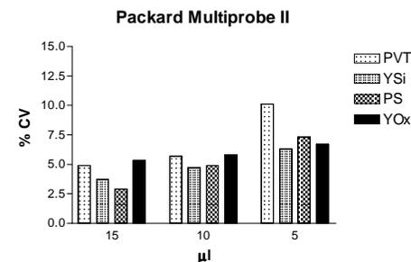
Figure 2. Precision achieved when dispensing [<sup>3</sup>H] labelled beads into a 384 well plate using the Packard Multiprobe II.
