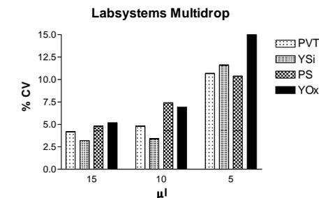
Figure 4. Precision achieved when dispensing [<sup>3</sup>H] labelled beads into a 384 well plate using the Labsystems Multidrop.
