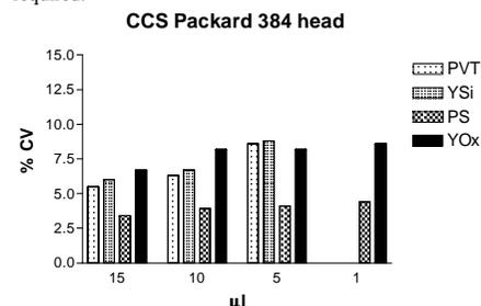
Figure 1. Precision achieved when dispensing [<sup>3</sup>H] labelled beads into a 384 well plate using the CCS Packard 384 head.
