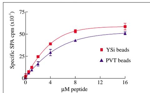
Figure 5. Specific SPA cpm as a function of peptide concentration using both YSi and PVT his-tag SPA beads. 0.5 $\mu$ M to 16 $\mu$ M peptide was incubated with 10mU CKII enzyme for 30 minutes at 37°C. 500 $\mu$ g YSi and 1mg PVT beads were used to capture the product.
