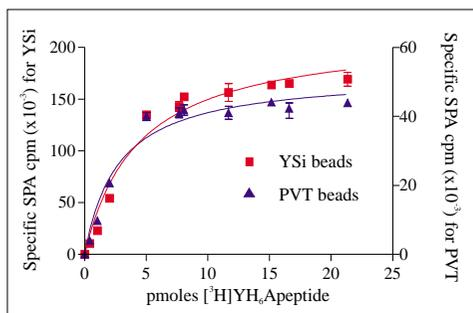
Figure 2. Saturation binding for YSi and PVT his-tag beads with [<sup>3</sup>H]Y(H)<sub>6</sub>A peptide using 10 $\mu$ g bead per well. All data points in this and subsequent figures are means of 3 replicates.
