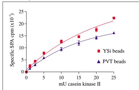
Figure 4. CKII enzyme concentration dependency using both YSi and PVT his-tag SPA beads and a range of 1mU to 25mU enzyme. Incubation was for 30 minutes at 37°C.
