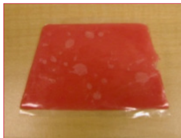
Figure 1. Picture of the fiber filled dental resin used for the UV curing experiment
