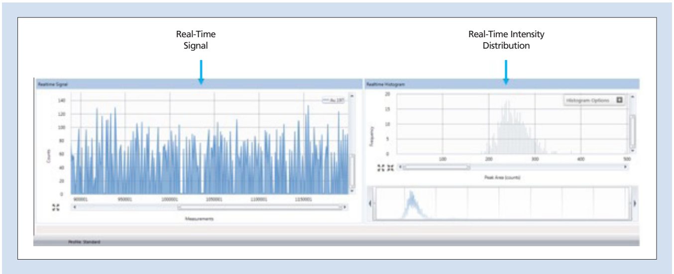
Figure 5. A snapshot of the Analysis panel taken during acquisition showing both the real-time data (zoomed-in to show individual pulses) and the real-time distribution histogram.
