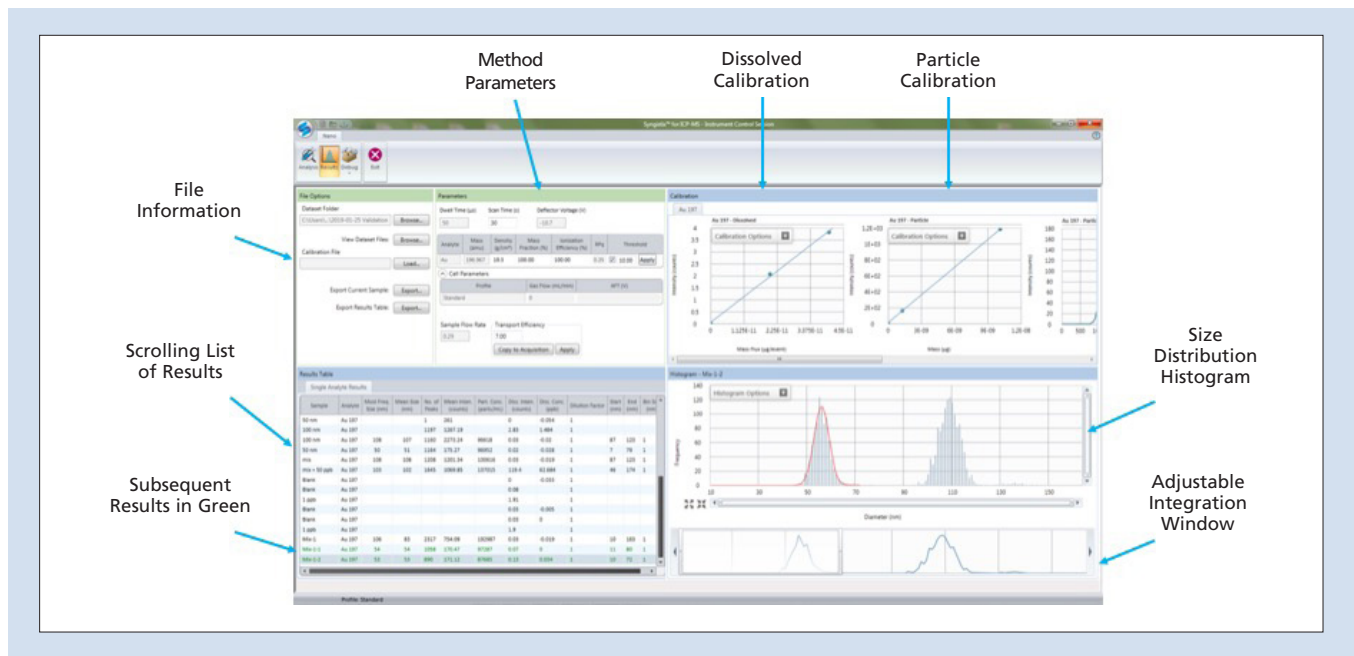
Figure 6. The Results panel, featuring reprocessed data saved as subsequent results in green color.
