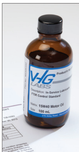
Figure 2. In-Service Lubricants FT-IR oil
