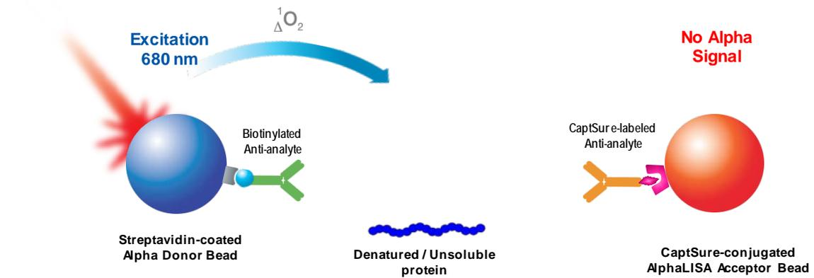
**Figure 2 : Principle of detection of the soluble protein by the Alpha SureFire® CETSA® assay. Only the soluble protein will lead to the generation of an Alpha signal (A), while the thermally denatured insoluble protein is unable to create the proximity needed for the generation of an Alpha signal (B).**
