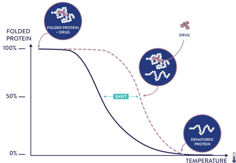
**Figure 1 : Principle of the CETSA<sup>®</sup> melting curve, and thermal stabilization by compound binding.**
