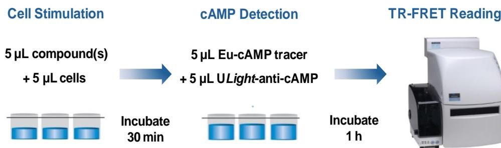
Figure 2. Standard assay procedure for the LANCE *Ultra* cAMP assay.
