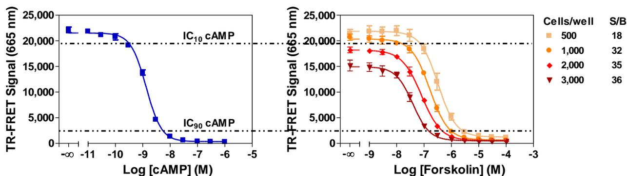
**Figure 5. Determination of optimal cell density.** Left panel: cAMP standard curve; right panel: cell and forskolin cross-titration. TR-FRET signal was measured with the EnVision Multilabel Plate reader set in laser mode.
