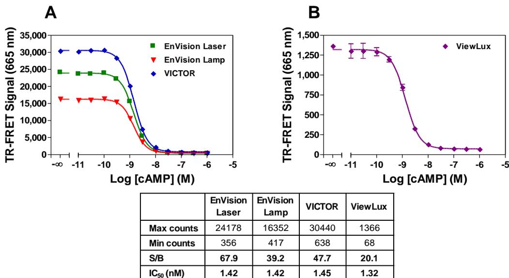
**Figure 3. Representative LANCE *Ultra* cAMP standard curves obtained on different TR-FRET readers.** Assay reagents were incubated in a white opaque OptiPlate™-384 microplate for 1 hour at room temperature. TR-FRET signal was detected with the (A) EnVision® Multilabel reader (laser and lamp settings), VICTOR™ reader and (B) ViewLux® CCD imager.
