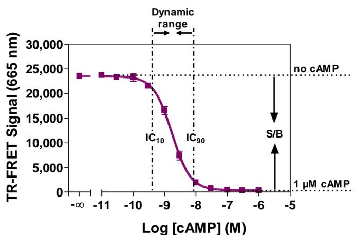
**Figure 4. Analysis of a LANCE *Ultra* cAMP standard curve obtained with the EnVision<sup>®</sup> Multilabel Plate reader set in laser mode.** This representative standard curve was analyzed with the GraphPad Prism<sup>®</sup> software using a sigmoidal dose response model with variable slope. In this example, signal-to-background (S/B) ratio was of of 70, with a ~1.5-log dynamic range (IC<sub>90</sub>-IC<sub>10</sub> values) and an IC<sub>50</sub> value of 1.4 nM..
