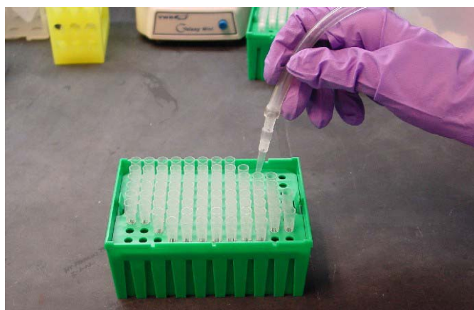
Figure 23. Replacing the disposable pipette tip.
