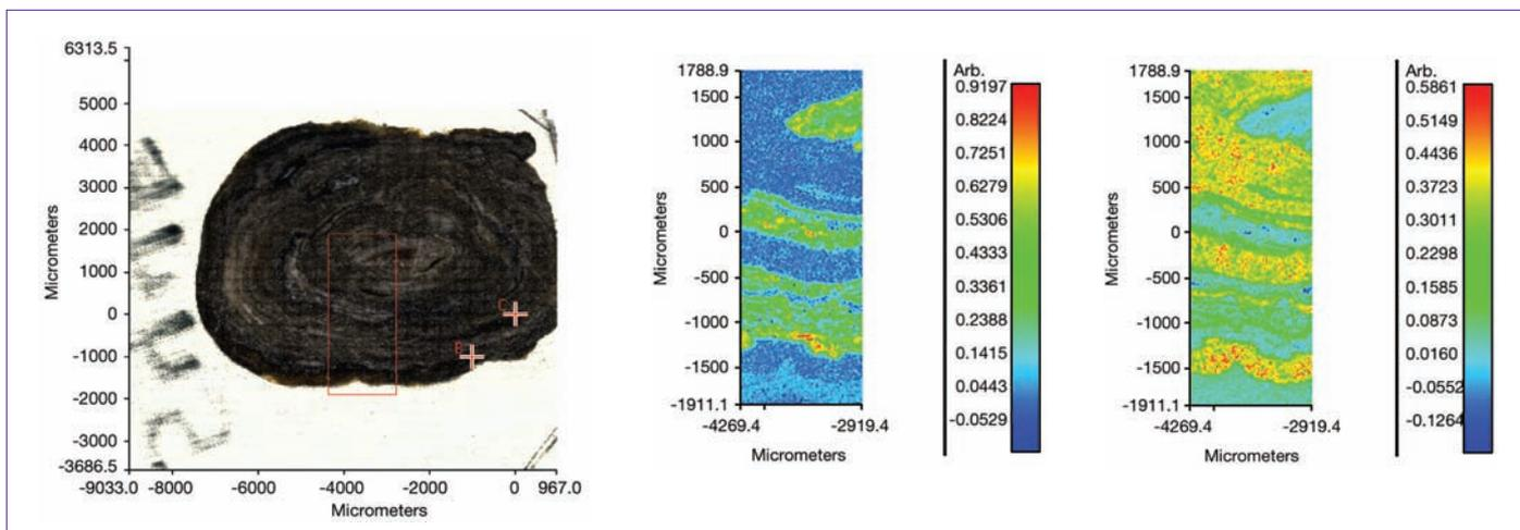
Figure 3. Visible and infrared images of a kidney stone.
