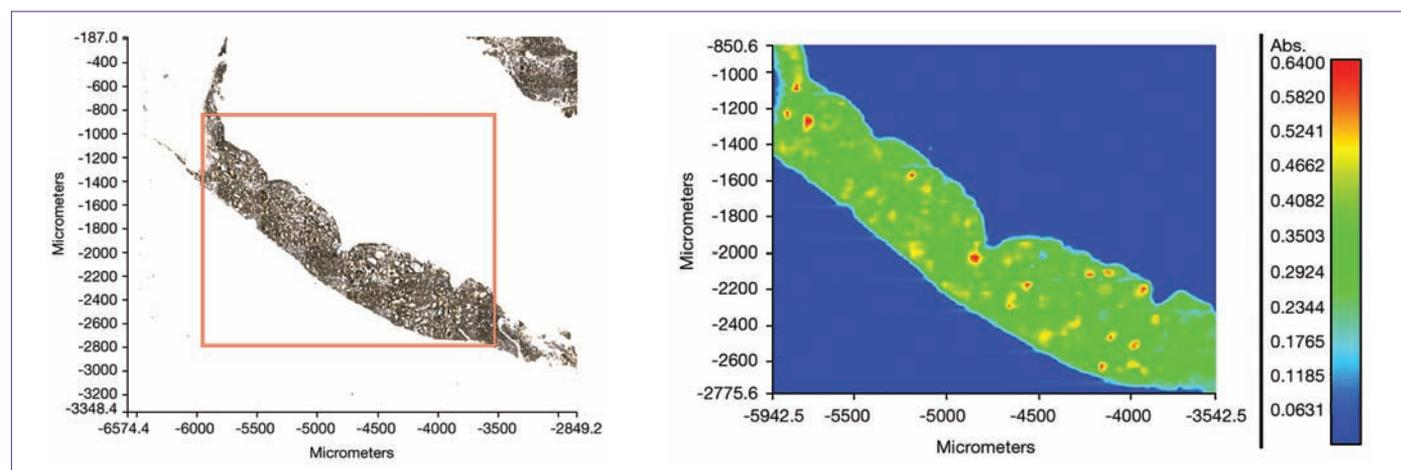
Figure 1. Visible and infrared image of thin section mounted on low-E glass.
