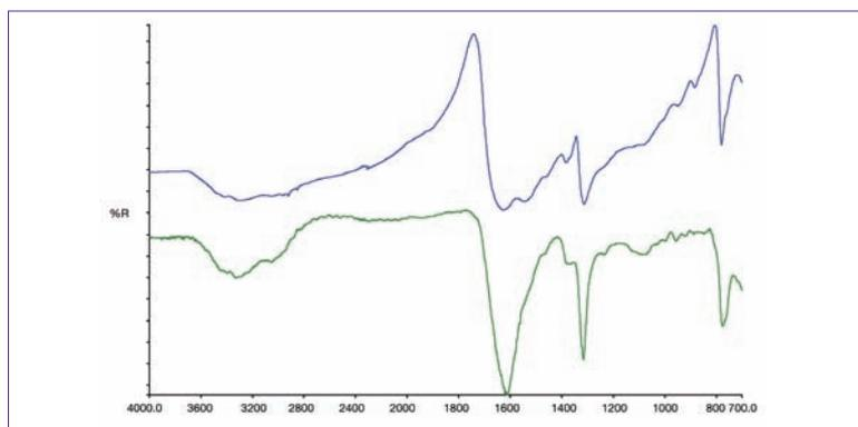
Figure 2. R/A (top) and ATR (bottom) spectra of mineral inclusion.
