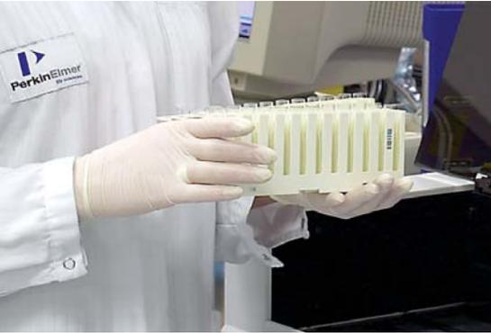
When you work with serum samples, up to 36 sample racks can be loaded at one time giving maximum capacity of 432 patient samples. Bar-coded primary tubes can be loaded directly. This reduces the need for sample transfer and helps to cut total costs.
