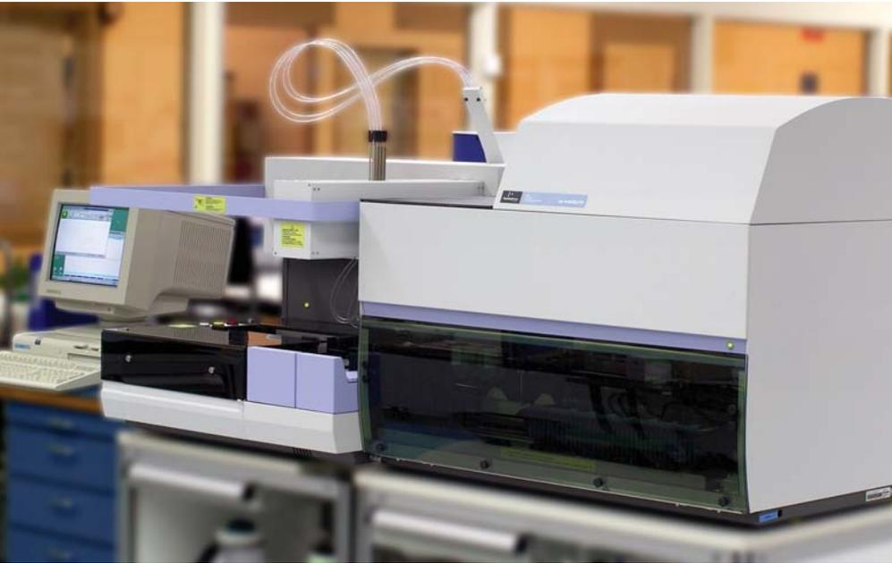
Within the AutoDELFI Plate Processor all assay stages including measurement are performed automatically.
