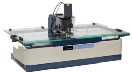
For dried blood spots the Sample Processor is replaced by a puncher “front end”. This punches filter paper disks of samples, standards and controls, and prepares the microplates for loading into the Plate Processor. PerkinElmer offers a choice of three puncher devices.
