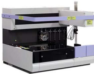
The Sample Processor unit accepts serum samples in primary or secondary sampling tubes. If sample dilution is needed, this is done automatically before the dispensing of sample, standard and control aliquots into microplates. The microplates are then automatically loaded into the Plate Processor unit.
