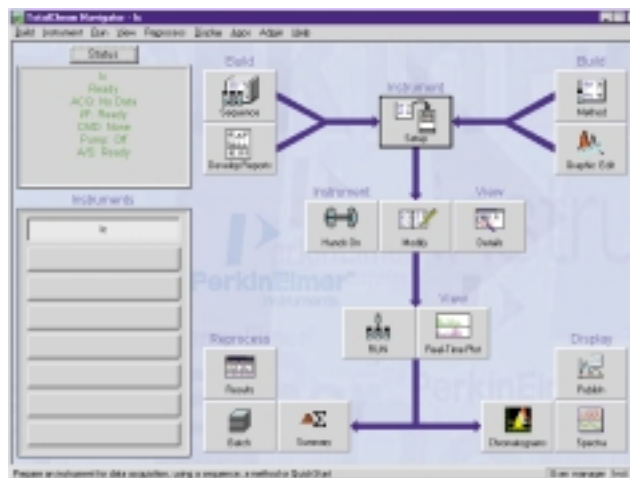
Figure 2. TotalChrom Navigator screen showing intuitive, icon-driven logic path for method development, instrument control and data processing.
