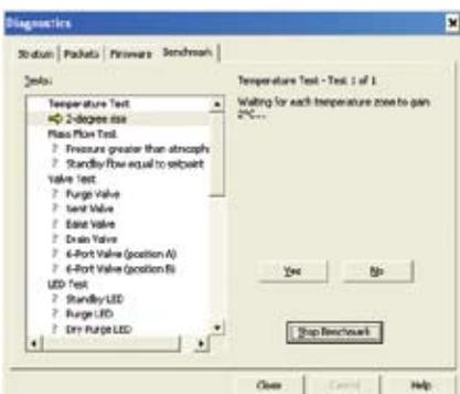
**Benchmark Screen** - The Benchmark screen contains an interactive program that tests heaters, LEDs, and the continuity of inputs and outputs on the CPU board. The results of the Benchmark Test are saved in the System History Log under the name entered before starting the benchmark.
