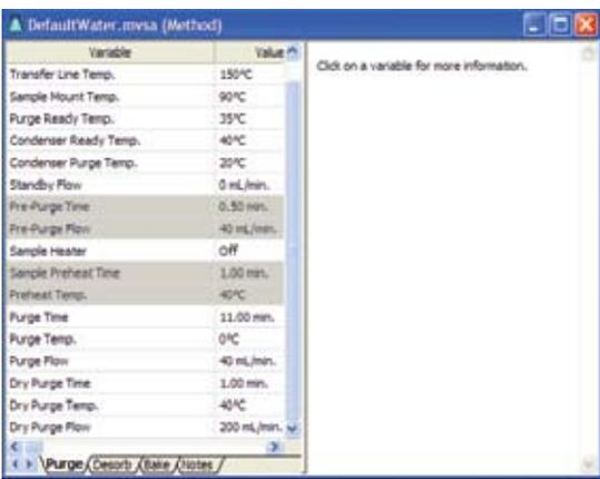
**Method Development Screen** - The Stratum TekLink™ Software comes pre-installed with methods for most applications. You can select one of these methods or if your application calls for a unique requirements, a customized method can be created to meet your analytical requirements for sample processing.
