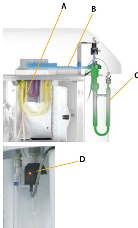
**A. Analytical Trap** - The Stratum PTC ships with a #9 proprietary U-shaped trap installed and a U-shaped Vocab 3000 trap. If a sample is not properly desorbed from the trap, the resolution in the chromatogram will suffer. The U-shaped trap provides superior peak shape by allowing a volume for the desorbing gas to refocus before proceeding to the GC. The result is a dramatic improvement in your chromatographic resolution.
