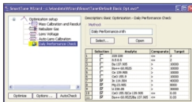
Figure 3. The SmartTune optimization wizard sets up user-defined optimization and performance-check procedures, automatically running them while you perform other tasks – maximizing your productivity.
