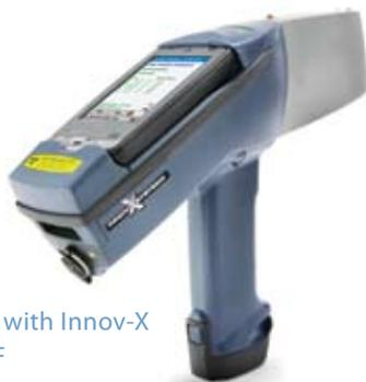
Metals Screening with Innov-X Import Guard XRF
