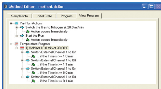
Figure 12. A typical UV curing method window. Note the parameters set by the user.
