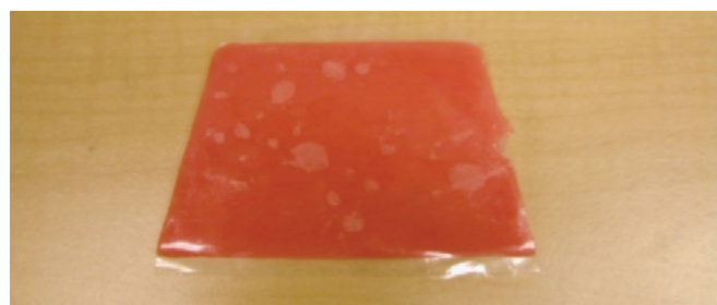
Figure 2. Picture of the fiber filled dental resin used for the UV curing experiment.
