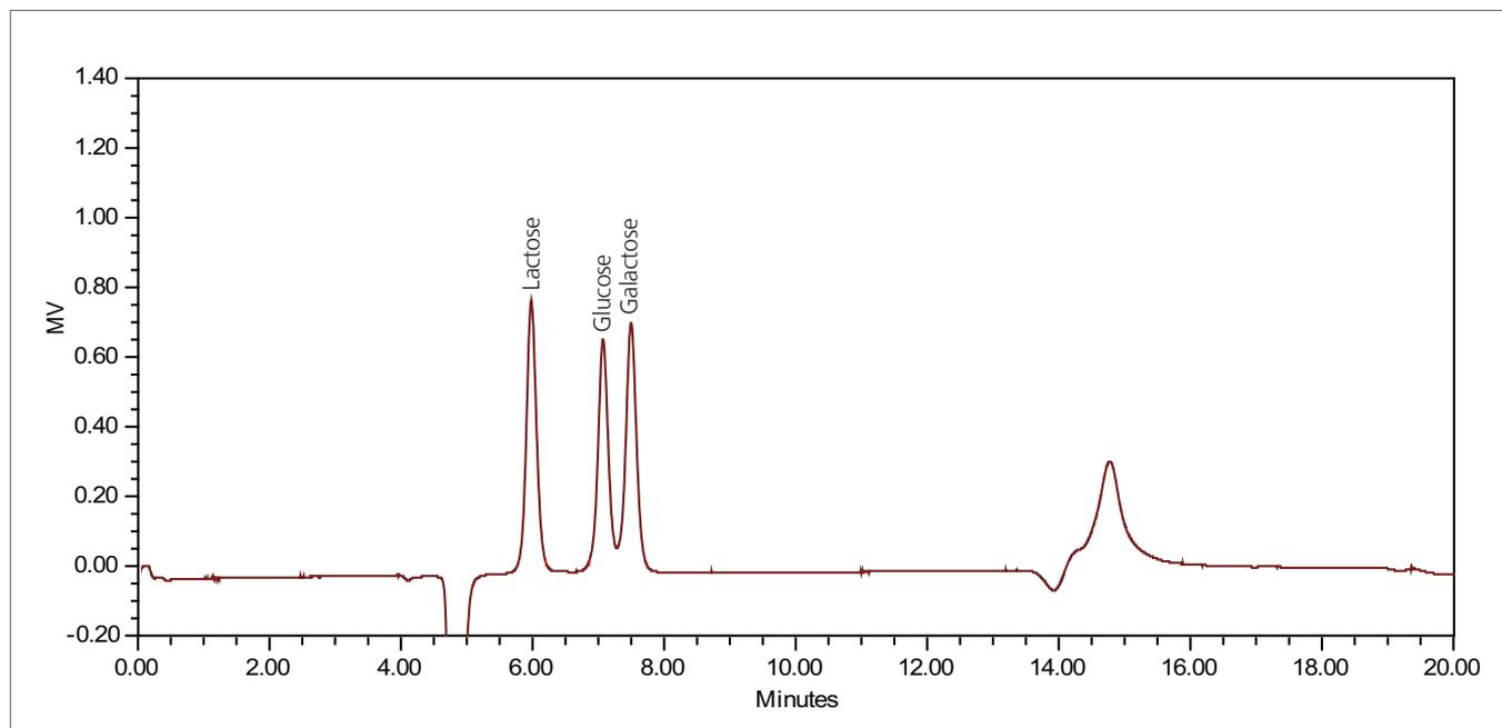
Figure 1. Chromatogram of the 0.005% (50 ppm) standard solution of lactose, glucose and galactose; 10- $\mu\text{L}$  inj.
