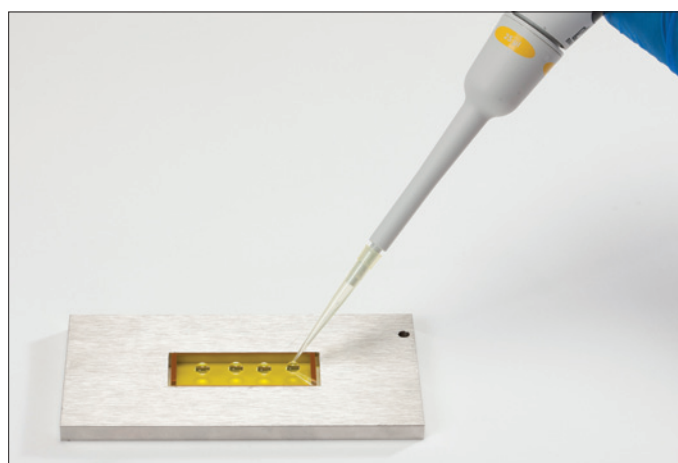
Figure 5. Sample deposition for the HATR method, constraining the sample to the most brightly illuminated portion of the crystal.
