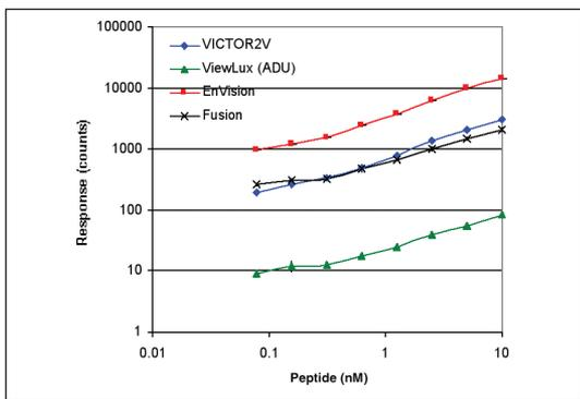
Figure 7. LANCE instrument performance for peptide dilution series measured with black OptiPlate-384.
