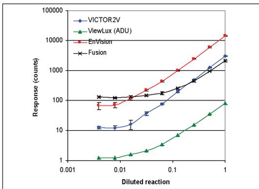
Figure 8. LANCE instrument performance for diluted reaction measured with black OptiPlate-384. X-axis presents the dilution factor where 1 is composed of 10 nM peptide, 50 nM SA-APC and 1 nM Eu-labeled anti-P-Tyr antibody diluted in the assay buffer and where 0.1 corresponds components diluted 1:10 in the reaction buffer.
