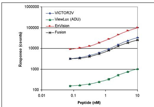
Figure 5. LANCE instrument performance for peptide dilution series measured with white OptiPlate-384.
