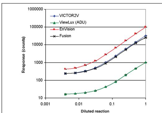
Figure 6. Instrument performance in LANCE for diluted reaction measured with white OptiPlate-384. X-axis presents the dilution factor where 1 is composed of 10 nM peptide, 50 nM SA-APC and 1 nM Eu-labeled anti-P-Tyr antibody diluted in the assay buffer and where 0.1 corresponds components diluted 1:10 in the reaction buffer.
