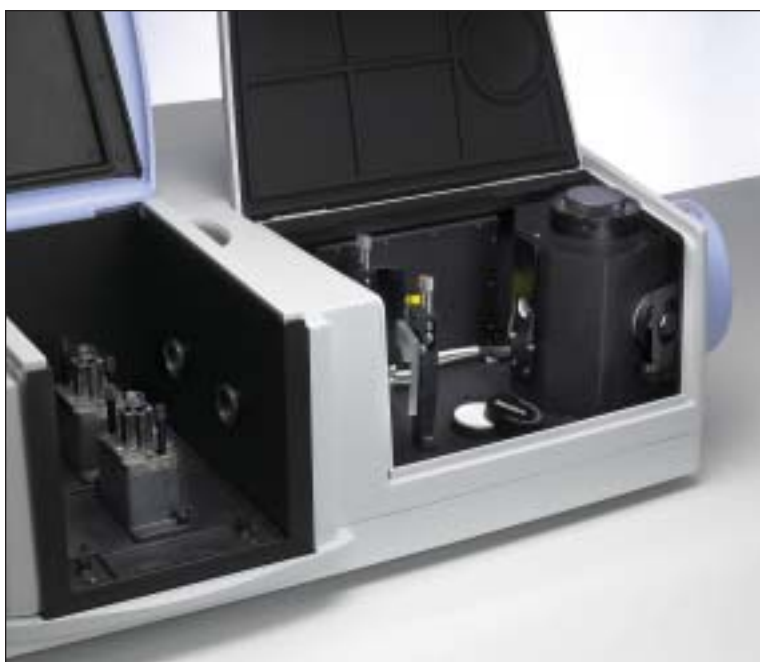
Figure 1. The dual sampling areas on the LAMBDA™ 650/850/950.
