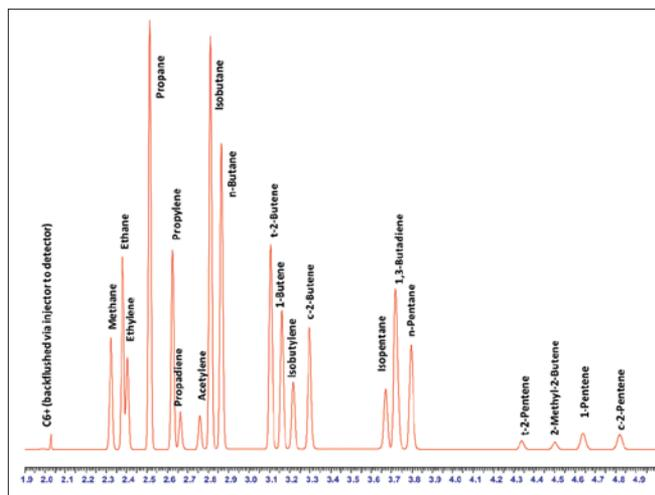
Figure 4. Expansion of a section taken from Figure 3 showing the analyte peaks.
