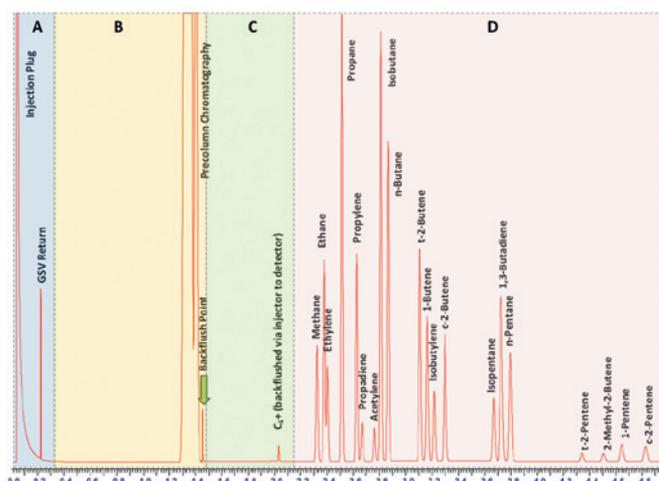
Figure 3. Chromatogram of a refinery gas standard mixture.
