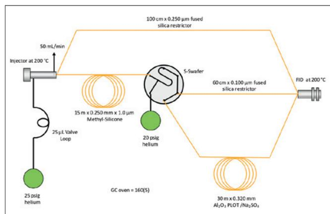
Figure 1. S-Swafer configuration to enable the backflush point to be established and the precolumn effluent to be directed to a detector.
