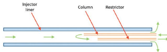
Figure 2. Positioning of the ends of the column and restrictor tube inside the injector liner.
