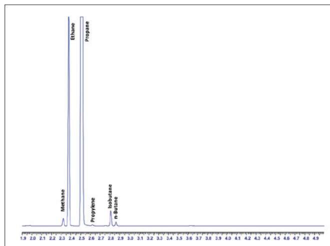
Figure 5. Chromatogram of liquid petroleum gas.
