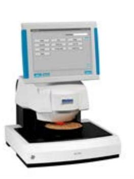
The instrument is handled by an intuitive touch screen interface and in less than 10 seconds samples are measured in flexible open dishes. Most sample types can be measured as they are without any preparation or as an alternative be grinded and measured as powder or coarse meal.
