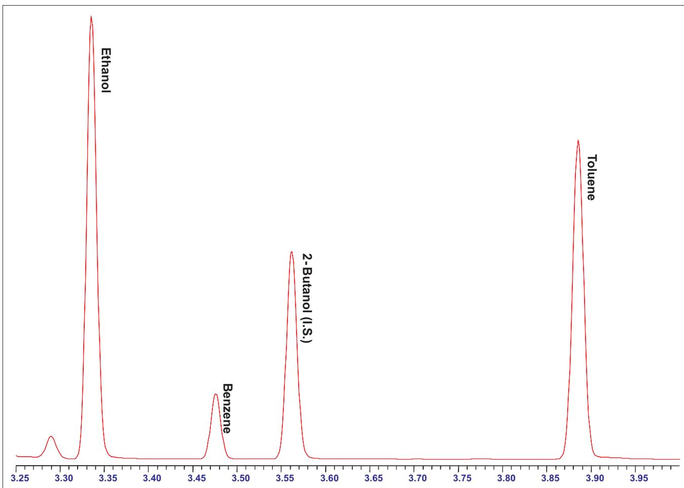
Figure 9. Chromatography of a typical gasoline sample with 2-butanol added as an internal standard.
