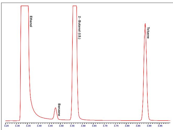
Figure 10. Chromatogram of standard mixture containing 0.05% v/v benzene and 0.5% v/v toluene in pure ethanol with added internal standard.
