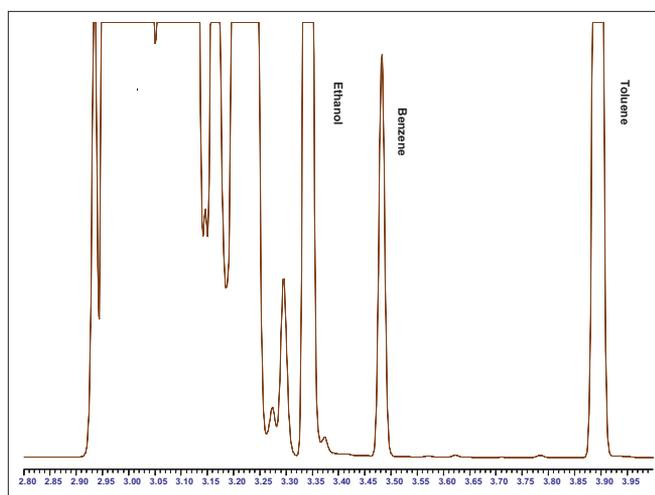
Figure 7. Chromatography eluting from the TCEP column for a typical gasoline sample with a timed event to reduce the injector pressure and increase the midpoint pressure at 1.61 minutes.
