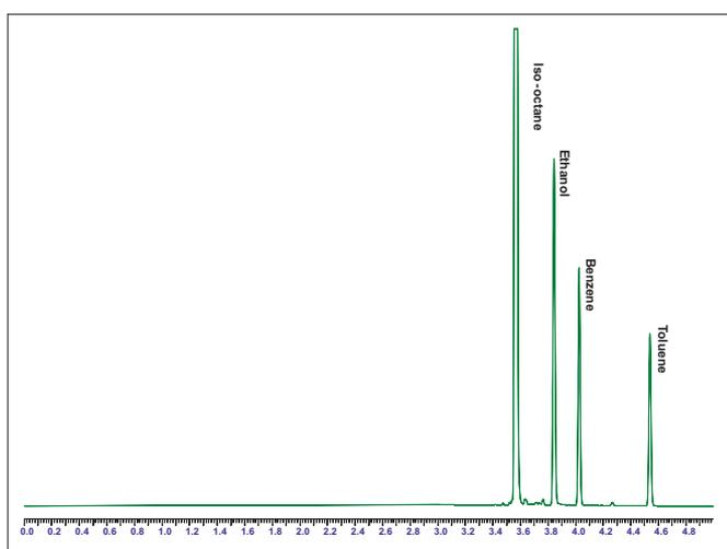
Figure 5. Chromatography of mixture eluting from TCEP column.
