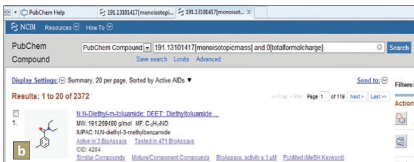
Figure 4 a and b. Accurate mass and isotope ratio of unknown analyte was entered into AxION EC ID software to determine elemental composition. The AxION EC ID software searches against the PubChem database and by sorting for decreasing AIDs (chemical listed for most number of assays), the first possible candidate for the given elemental composition was given as N, N-Diethyl-m-toluamide (DEET), a common ingredient in insect repellents.
