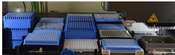
Figure 7. Deck layout after the second pause in the module, when the PCR mastermix is added to the deck
