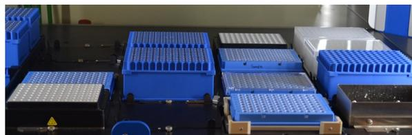
Figure 8. Deck layout for SPRI cleanup module
