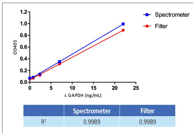
Figure 1. Linear regression generated from the optical density – GAPDH concentration relation for the spectrometer and filter mode absorbance measurements together with the R<sup>2</sup> values.
