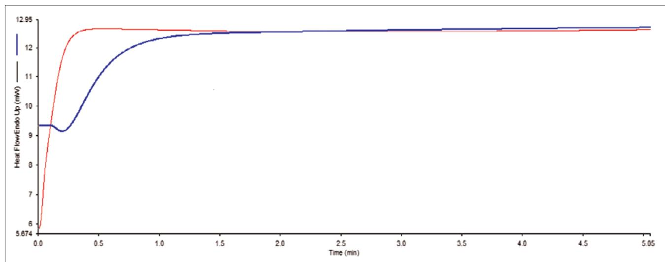
Figure 2. Example of startup transition of double-furnace DSC (red) and single-furnace heat flux DSC (blue) with the same experimental condition.
