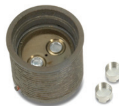
Figure 2. The double-furnace design pictured on the right allows very fast cooling and heating required for isothermal crystallization studies.
