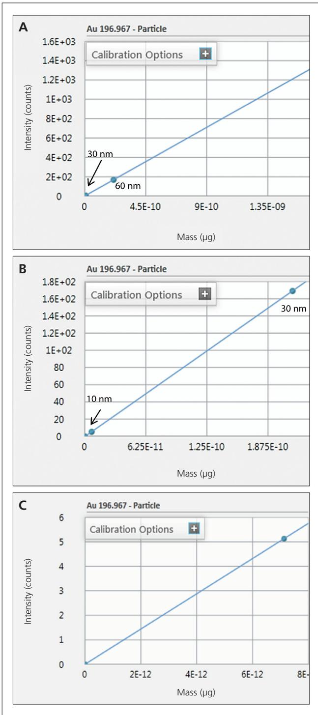
Figure 2. Particle calibration for 10, 30, and 60 nm Au NPs (A); Zoomed-in particle calibration showing 10 and 30 nm Au NPs (B); Zoomed-in particle calibration showing 10 nm Au NP and origin (C).
