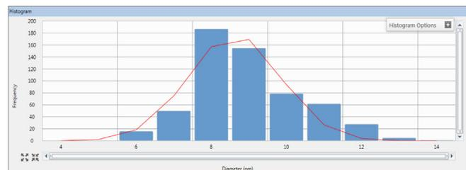
Figure 4. Particle size distribution for NIST 8011 10 nm Au NPs, fitted with a Gaussian distribution.
