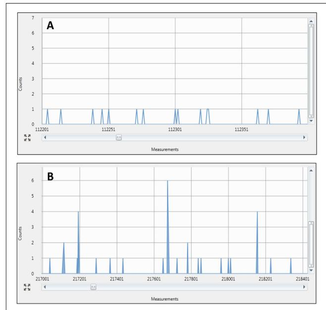
Figure 3. Real-time trace for a blank (A) and 10 nm Au NPs (B), with the x-axis zoomed so that individual acquisition points can be seen.
