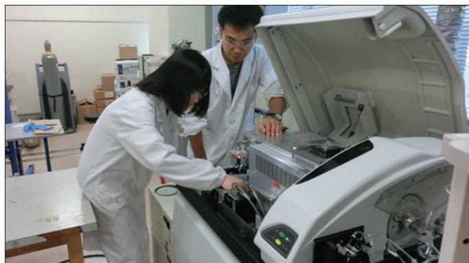
Dr. Takagai teaches his students at Fukushima University how to operate the ICP-MS with a broad range of detection limits, to test for contaminants in soil, water and food samples.
