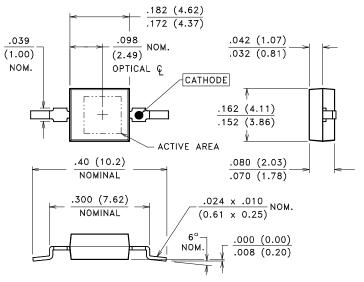
CASE 22 MINI-DIP (SURFACE MOUNT) CHIP SIZE: .120 x .120 (3.05 x 3.05) EXPOSED ACTIVE AREA: .0115  $\operatorname{in}^2$  (7.42  $\operatorname{mm}^2$ )
