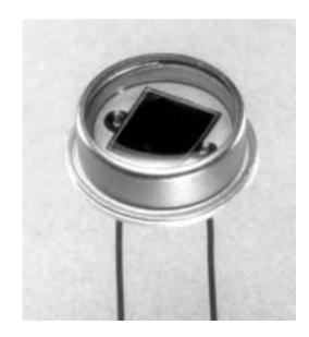
Large area planar silicon photodiode in a dual lead TO-8 package with a UV transmitting "flat" window. Cathode is common to the case. These diodes have very high shunt resistance and have good blue response.
