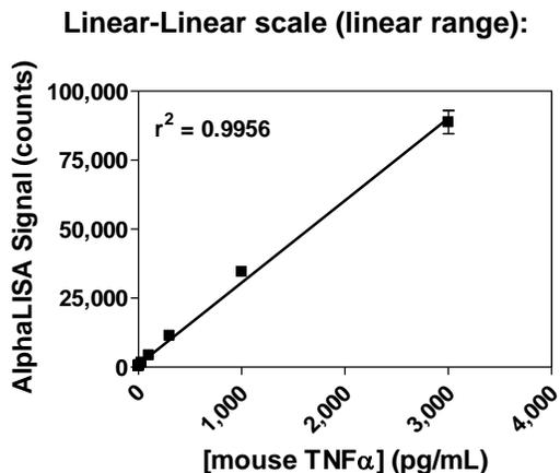
The data was generated using a white Optiplate-384 microplate and an EnVision-Alpha Reader 2102.
