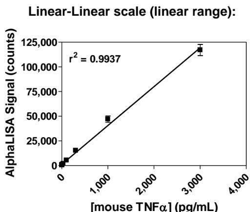
The data was generated using a white Optiplat-384 microplate and an EnVision-Alpha Reader 2102.
