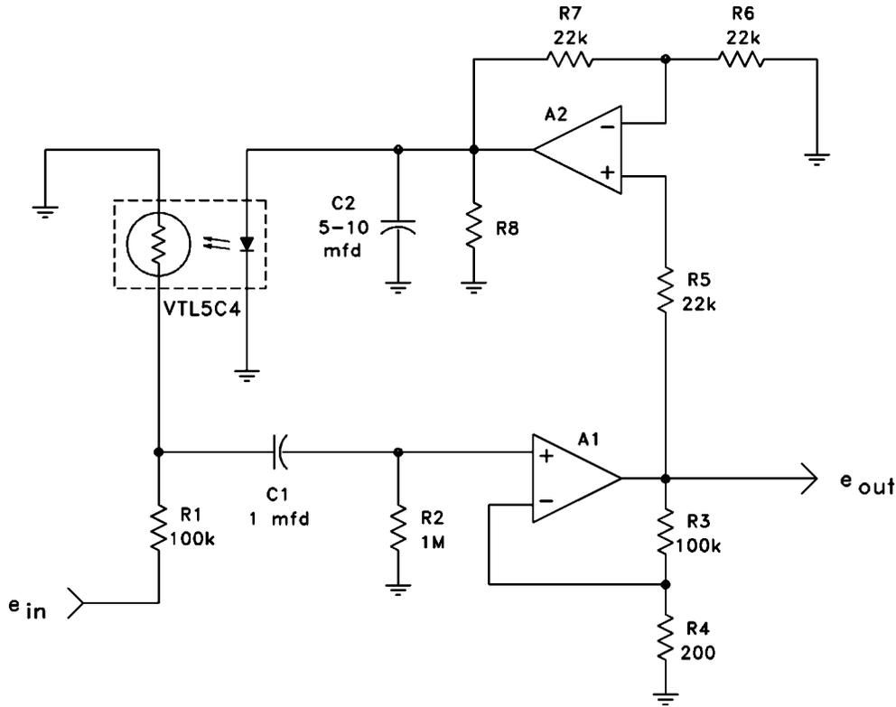
Figure 5. Peak Sensing Compressor with Constant Bandwidth
