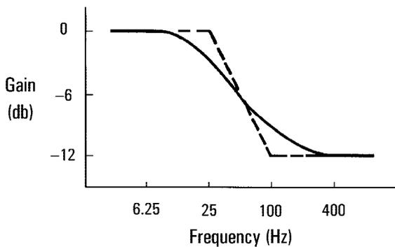
Figure 8b. Amplitude vs. Frequency for the Amplifier
