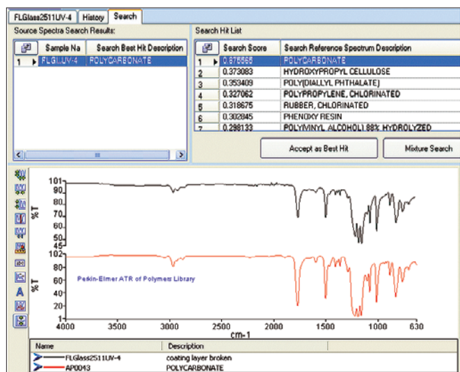
Figure 7. Search results for the headlight cover, showing a good match against the Polycarbonate reference.
