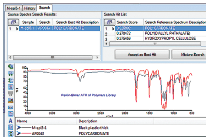
Figure 10. Sample 2 identified as Polycarbonate base material.
