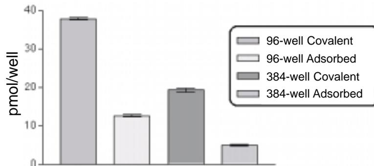
**Figure 2:** Biotin binding capacity comparison for adsorbed and covalent coated streptavidin FlashPlates. [<sup>3</sup>H]Biotin tracer at 300 pmol/ml, 200  $\mu$ l/well for 96-well plates and at 800 pmol/ml, 50  $\mu$ l/well for 384-plates. [<sup>3</sup>H]Biotin binding was determined by LSC quantitation of unbound tracer.
