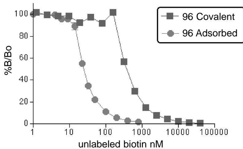
**Figure 1:** Competition curve of 5 pmol/ml [<sup>3</sup>H]biotin tracer with added unlabeled biotin. Binding comparison of adsorption and covalent coated streptavidin FlashPlates. The 50% inhibition of tracer binding (IC<sub>50</sub>) by unlabeled biotin was 300 pmol/ml for a 96-well plate and 500 pmol/ml for a 384-well plate (data not shown).
