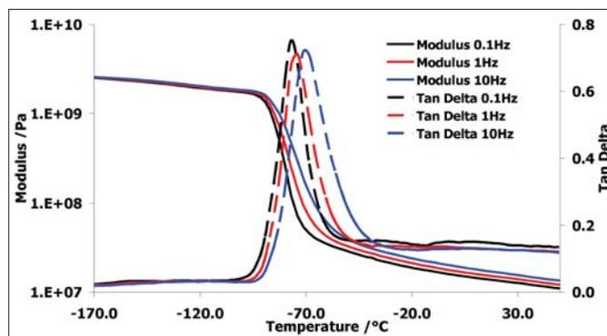
Figure 1. Glass transition of polybutadiene rubber.
