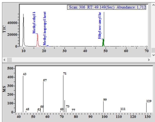
Figure 1. Chromatogram and mass spectrum, with identification of marker components in a Euro spike of a blended Scotch Whisky
