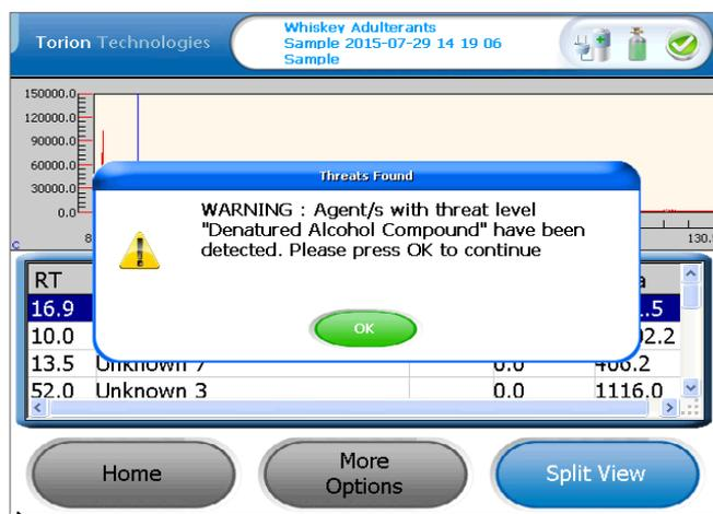
Figure 2. An example of an 'Alert' when a target compound in denatured alcohol is detected.
