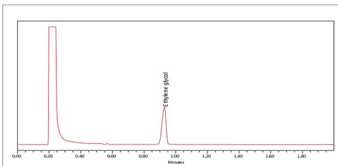
Figure 1. Chromatogram shows elution of ethylene glycol.
