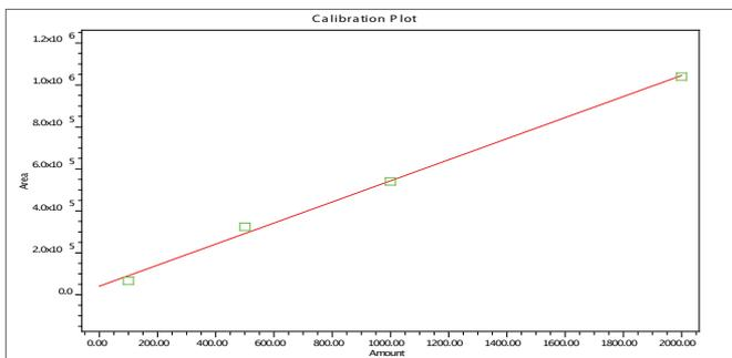
Figure 2. Calibration curve of ethylene glycol.
