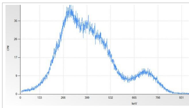
**Figure 2.**  $\alpha$ -spectrum after extraction of <sup>222</sup>Rn from a standard sample with Ultima Gold F in glass vials.
